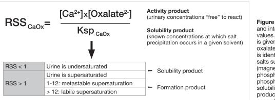
Figure 2. Calculation and interpretation of RSS values. The example is given for calcium oxalate, but the principle is identical for other salts such as struvite (magnesium ammonium phosphate) or calcium phosphate. Only solubility and formation products can vary according to the salt.
